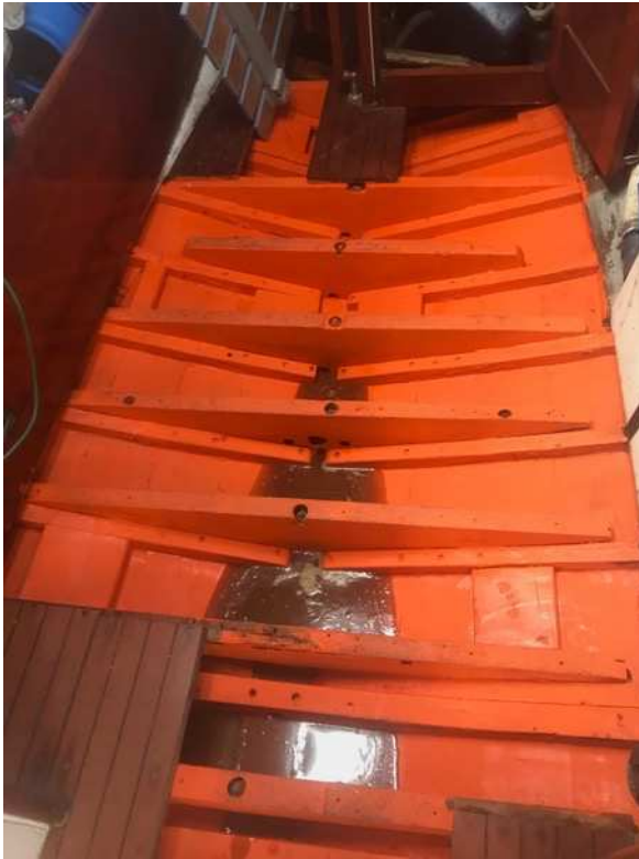
Main bilge after keel floor and frame heel work spring 2021
